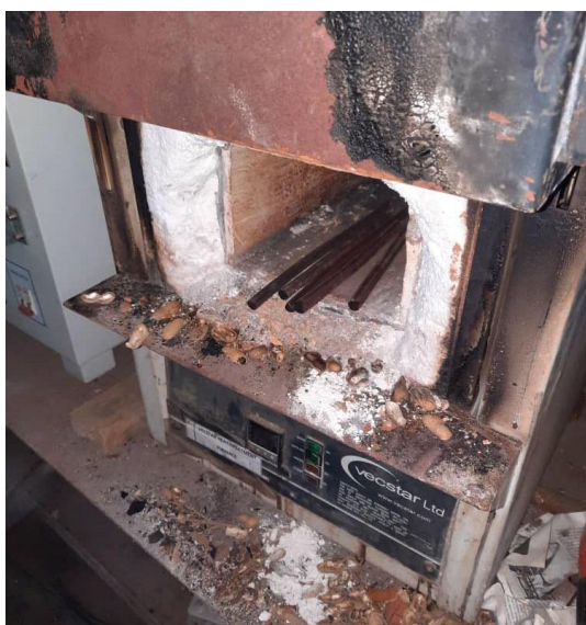
Fig 3: Specimen in Furnace before cold rolling
